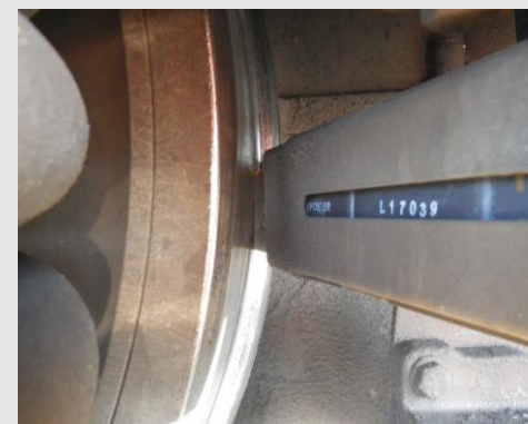
LCF solid stick on-board lubricant
