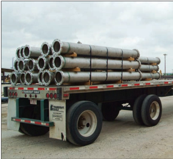
Stainless steel flanged column manufactured for water systems.
