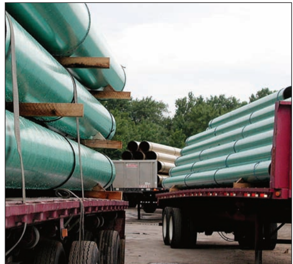
Fusion bond epoxy protective coating on steel line pipe.
