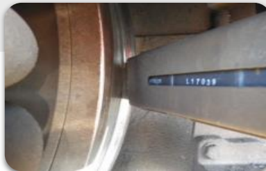
LFC Solid Stick On-Board Lubricant
